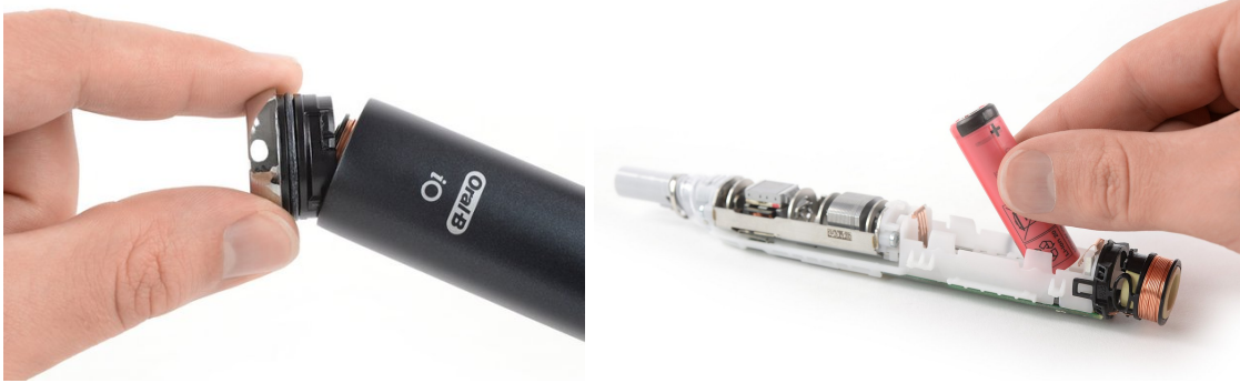
Fig. 2 and 3: removing the bottom cap of an Oral-B iO toothbrush (o-ring is visible) and removing the battery (image © iFixit)
