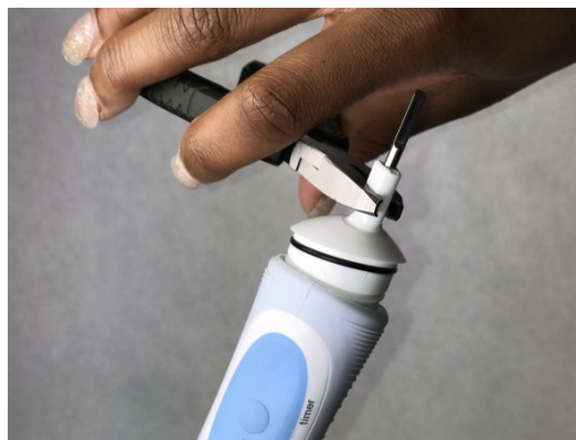
Fig. 4: removing the top cap of an Oral-B Vitality toothbrush (o-ring is visible) (image © iFixit)
